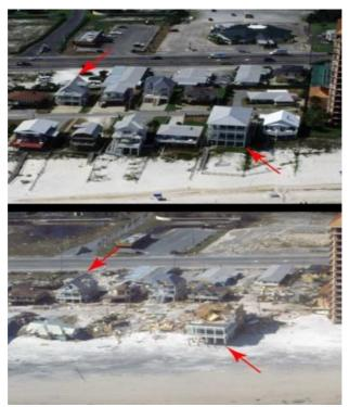
**Picture 3**. Results of a storm surge produced by Hurricane Katrina's strike - Orange Beach, Alabama. Image by USGS (the arrows show the specific buildings before and after the storm) [7].
