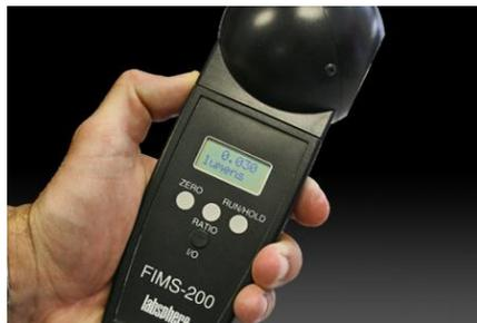
**Image 1.** Example of a simple photometer by Pro-Lite Technology
