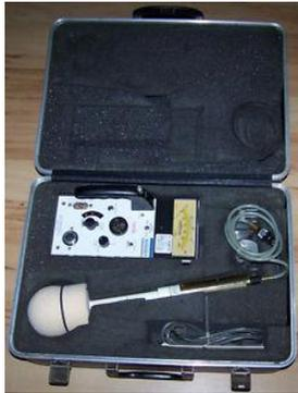
**Image 4.** Example of the electromagnetic field meter by Narda.
