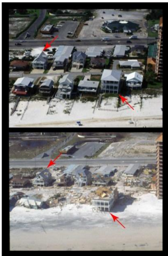
Ritratt 3. Results of a storm surge produced by Hurricane Katrina's strike - Orange Beach, Alabama. Image by USGS (the arrows show the specific buildings before and after the storm).
